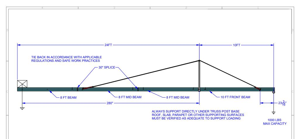
COUNTERWEIGHT OR CLAMP TO STRUCTURE TO PROVIDE RESISTANCE TO OVERTURNING WITH A SAFETY FACTOR OF 4 TO 1. REFER TO TABLE BELOW FOR REQUIREMENTS. USE COUNTERWEIGHT ADAPTERS TO SECURE ADDITIONAL WEIGHTS AS REQUIRED.
