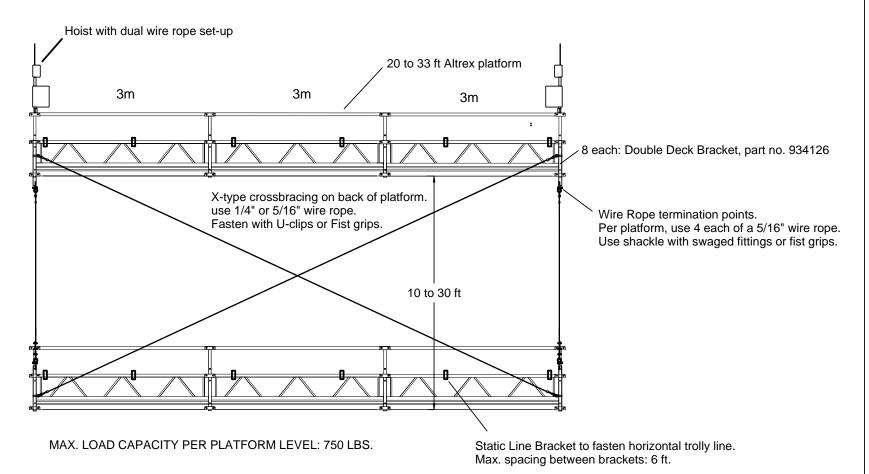
Horizontal trolly line is mandatory at the lower level(s). The workers on the upper level can choose between the trolly line or independent vertical lifelines.
