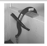
Similar to the Tank Top Roller, Ring Girder Rollers are used where a steel ring girder is located around a storage tank perimeter. Roller travels on rim of girder. It should be used in conjunction with hanging rope and tie back.
