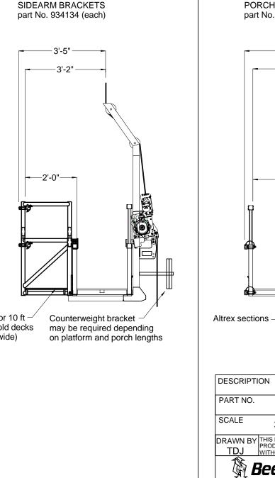
PORCH BRACKETS part No. 934127 (set of 2) 3'-11" 3'-7" 2'-5" Counterweight bracket may be required depending on platform and porch lengths Altrex porch options DATE 6/10/09 **REVISION NO.** 3/8"=1' DRAWN BY THIS DRAWING IS THE PROPERTY OF BEE ACCESS PRODUCTS AND IS NOT TO BE COPIED OR REPRODUCED WITHOUT THE CONSENT OF BEE ACCESS PRODUCTS. Bee Access Products
